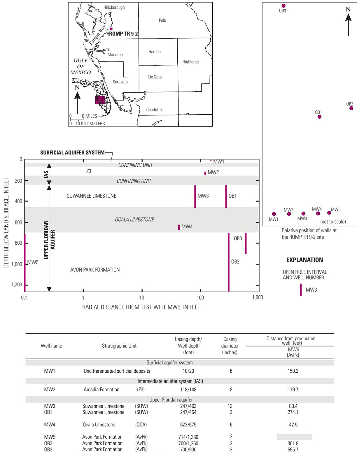
**Figure 42.** Generalized hydrogeologic section and location, plan view, description and configuration of wells at the ROMP TR 9-2 test site.
