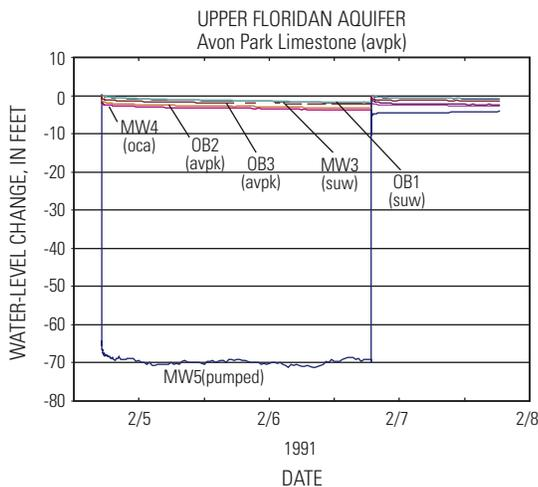
**Figure 43.** Water levels in selected wells during drawdown and recovery periods of the Avon Park aquifer test conducted at the ROMP TR 9-2 test site.
