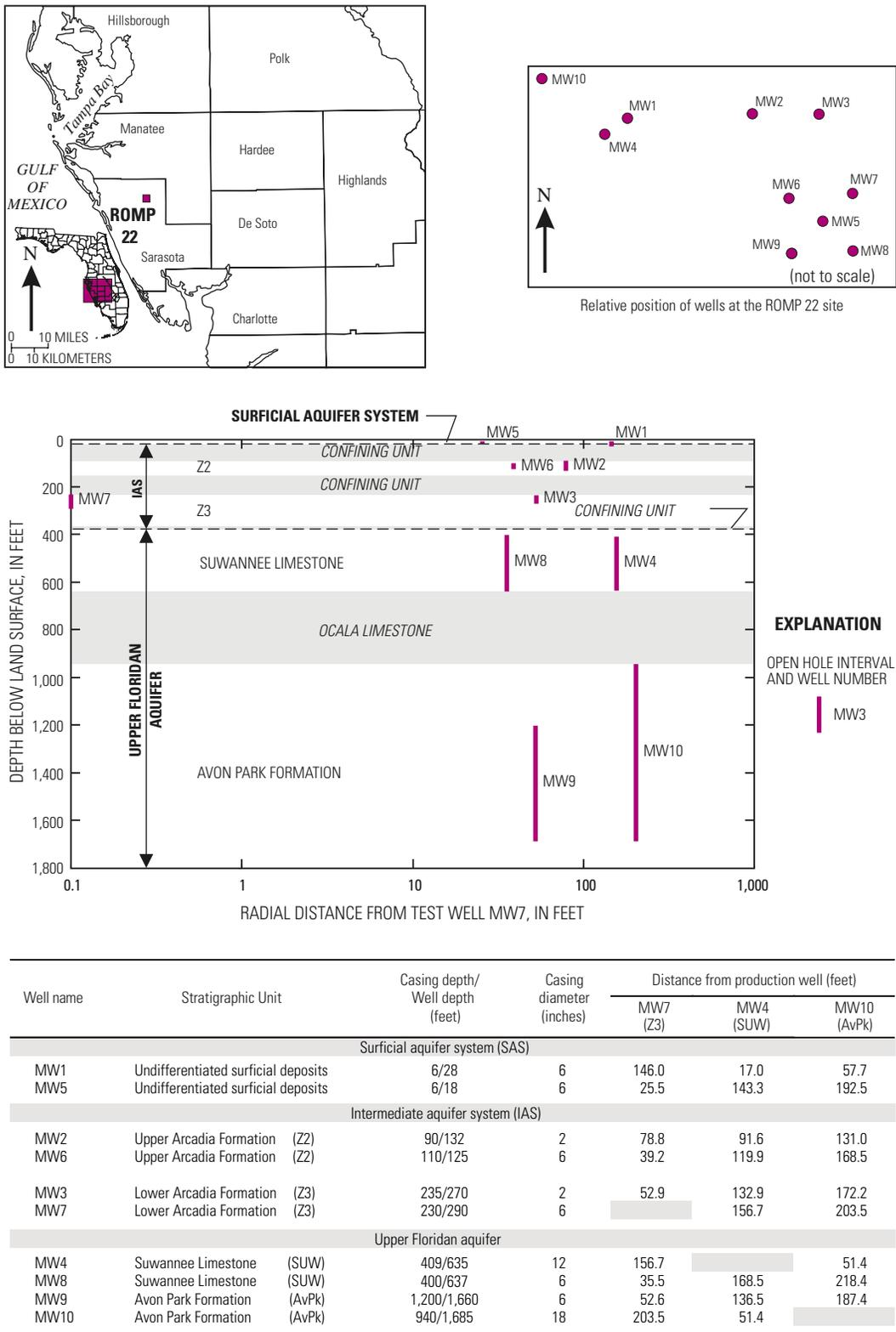
**Figure 26.** Generalized hydrogeologic section and location, plan view, description and configuration of wells at the ROMP 22 test site.
