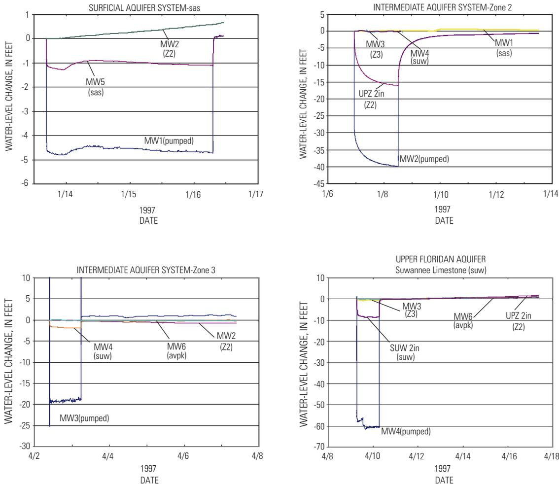
**Figure 7.** Water levels in selected wells during drawdown and recovery periods of the four aquifer tests conducted at the ROMP 5 test site.
