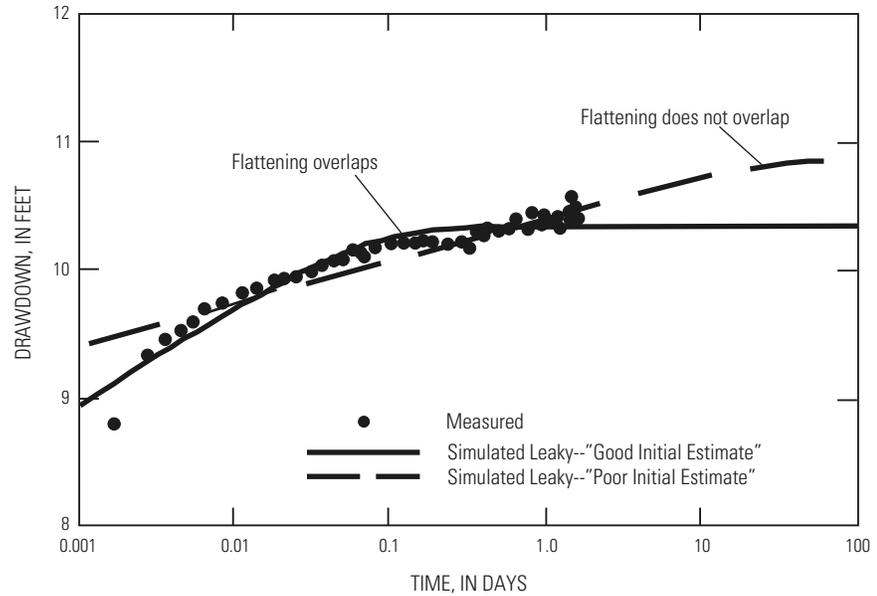
**Figure 4.** Effect of poor initial parameter estimates on model fit.
