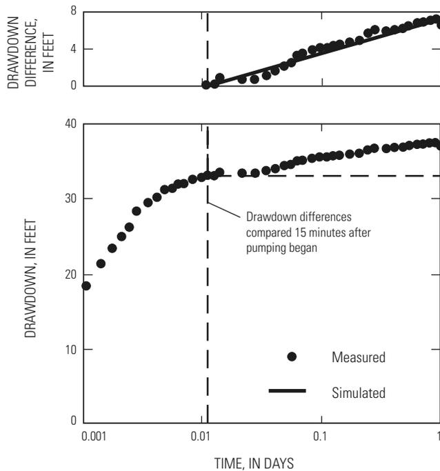
**Figure 5.** Effects of simulating drawdown in production wells after entry losses have stabilized.
