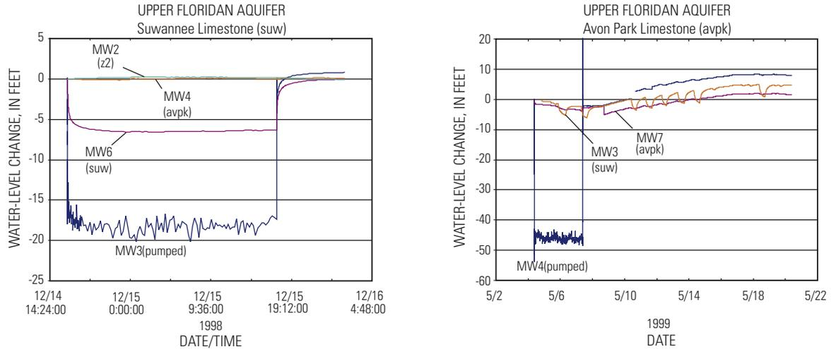
**Figure 30.** Water levels in selected wells during drawdown and recovery periods of the two aquifer tests conducted at the ROMP 25 test site.
