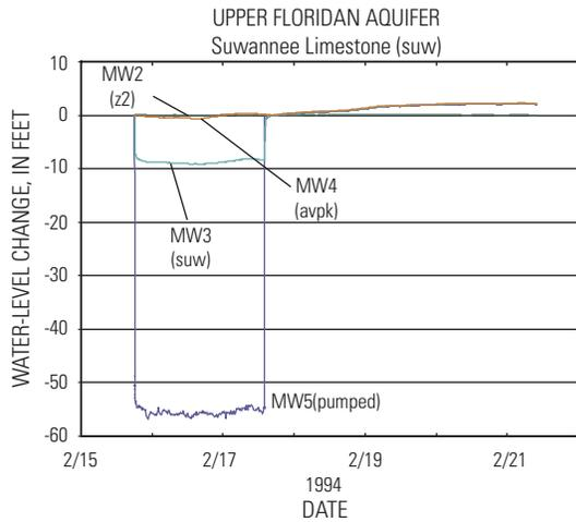
**Figure 37.** Water levels in selected wells during drawdown and recovery periods of the Suwannee Limestone aquifer test conducted at the ROMP 39 test site.
