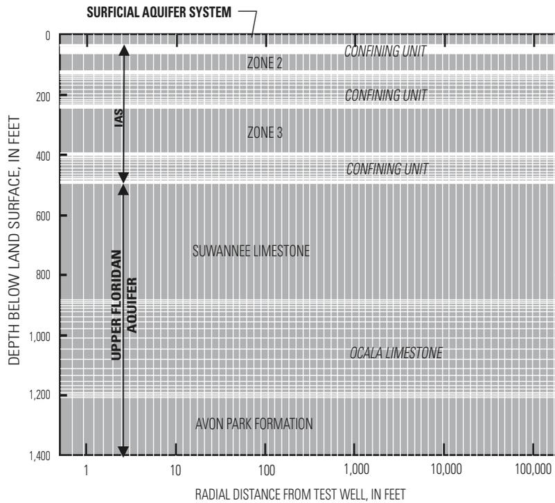
**Figure 3.** Hydrogeologic units and representative radial grid used for simulation of aquifer tests.
