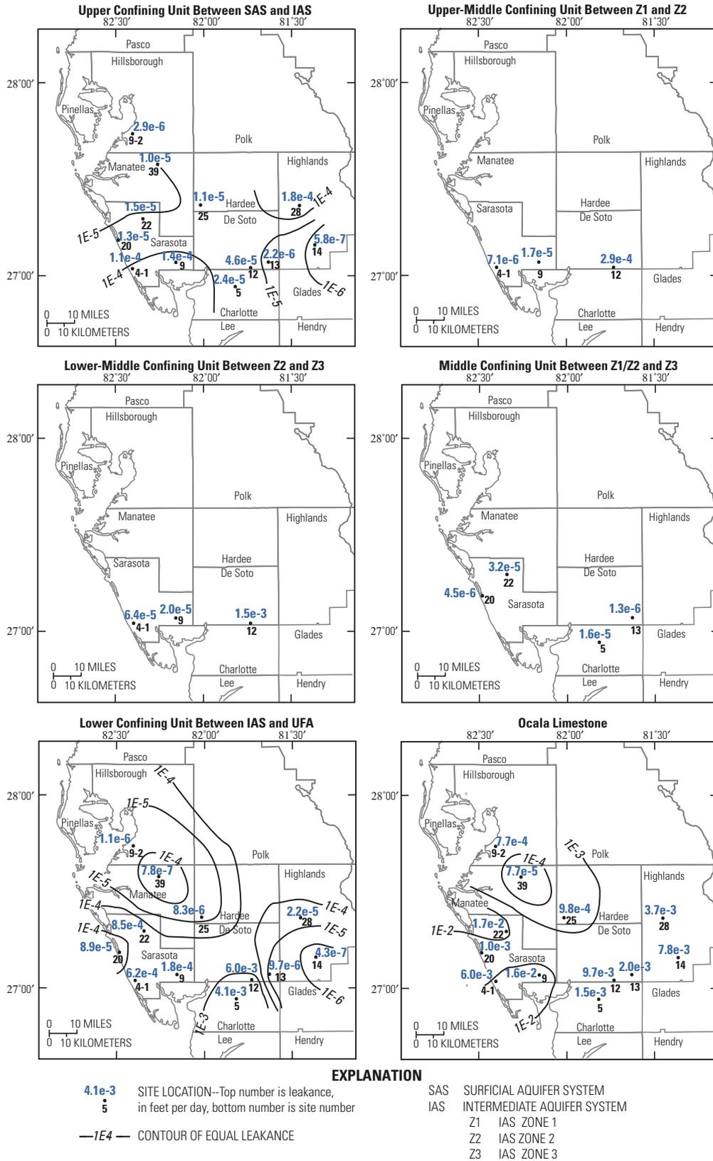
**Figure 48.** Distribution of leakance values estimated from numerical analyses of aquifer-test data collected at test sites.
