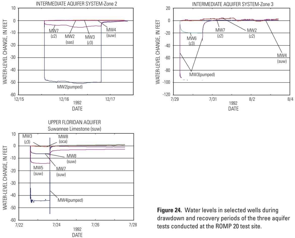
**Figure 24.** Water levels in selected wells during drawdown and recovery periods of the three aquifer tests conducted at the ROMP 20 test site.
