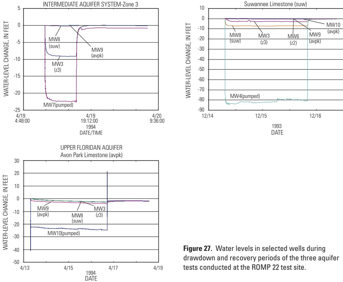
Figure 27. Water levels in selected wells during drawdown and recovery periods of the three aquifer tests conducted at the ROMP 22 test site.
