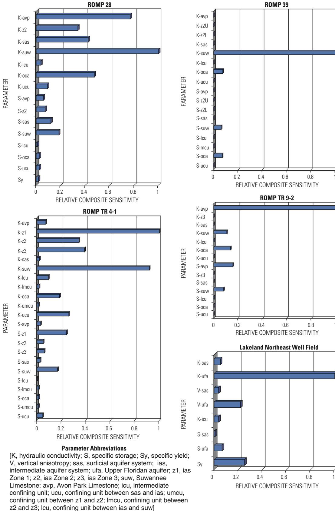
Figure 35. Relative composite sensitivity for final parameter values for ROMP 28, 39, TR 4-1, TR 9-2, and Lakeland Northeast Well Field.
