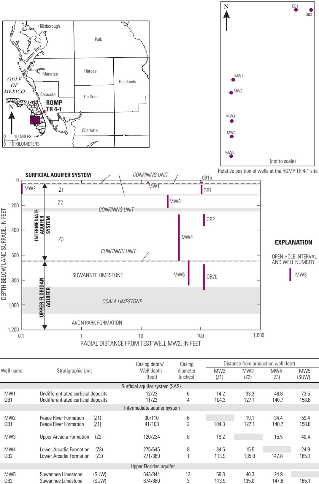
**Figure 39.** Generalized hydrogeologic section and location, plan view, description and configuration of wells at the ROMP TR 4-1 test site.
