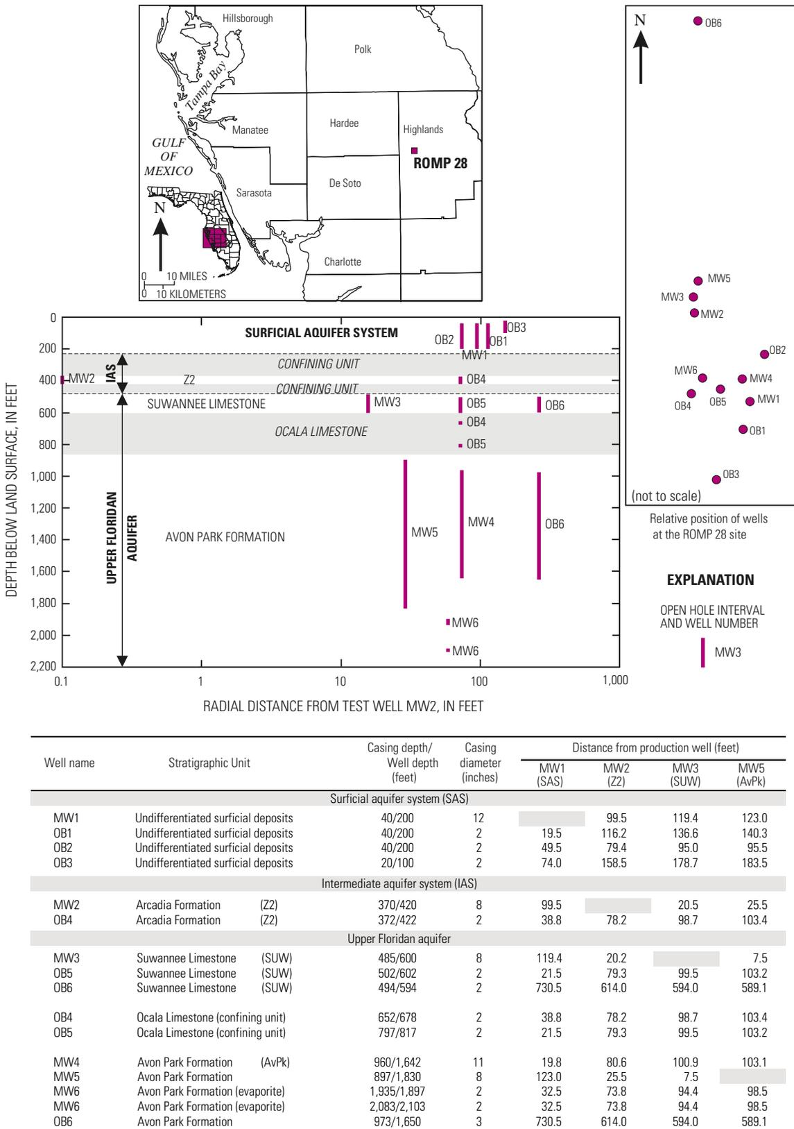
Figure 32. Generalized hydrogeologic section and location, plan view, description and configuration of wells at the ROMP 28 test site.
