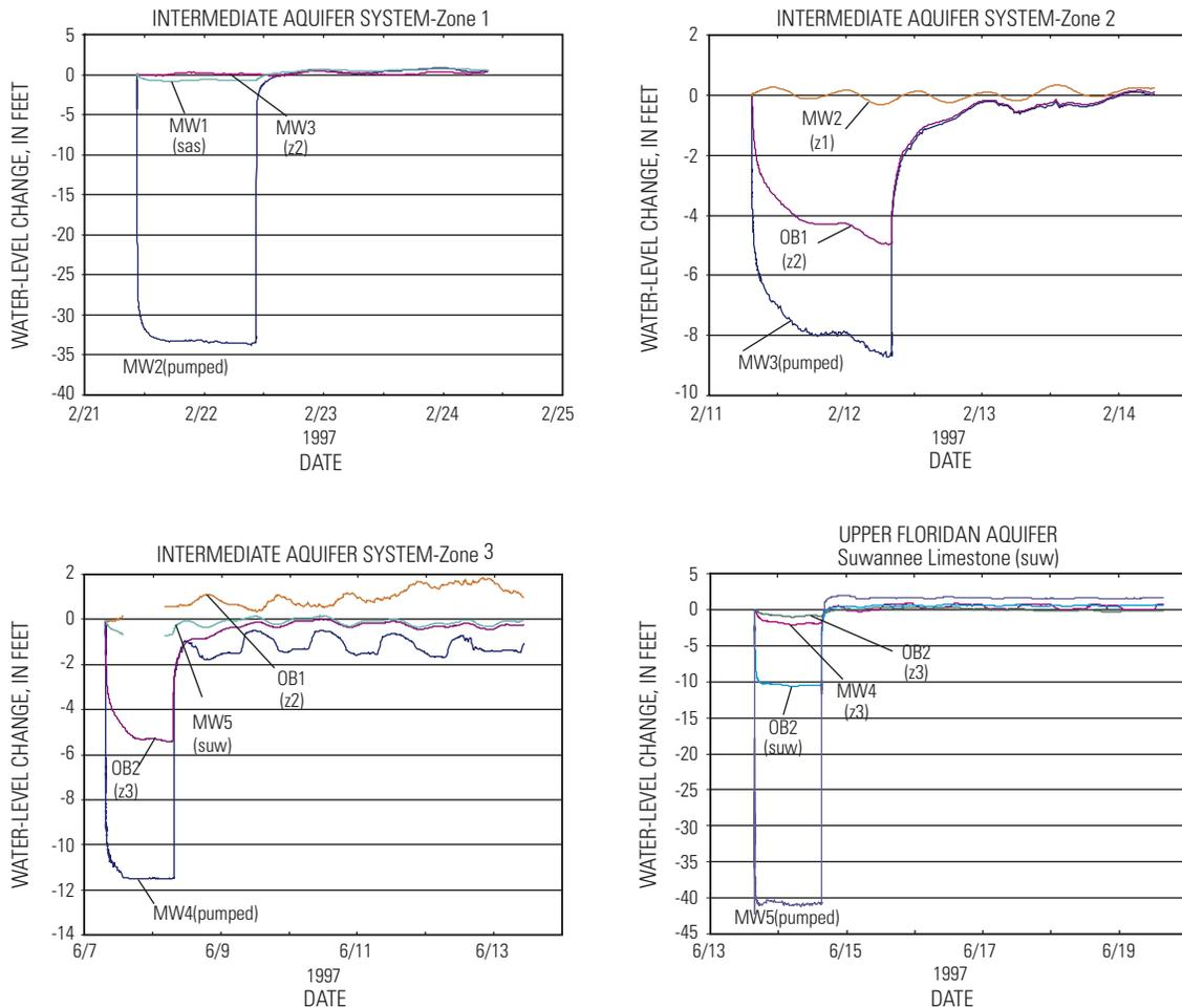
Figure 40. Water levels in selected wells during drawdown and recovery periods of the four aquifer tests conducted at the ROMP TR 4-1 test site.
