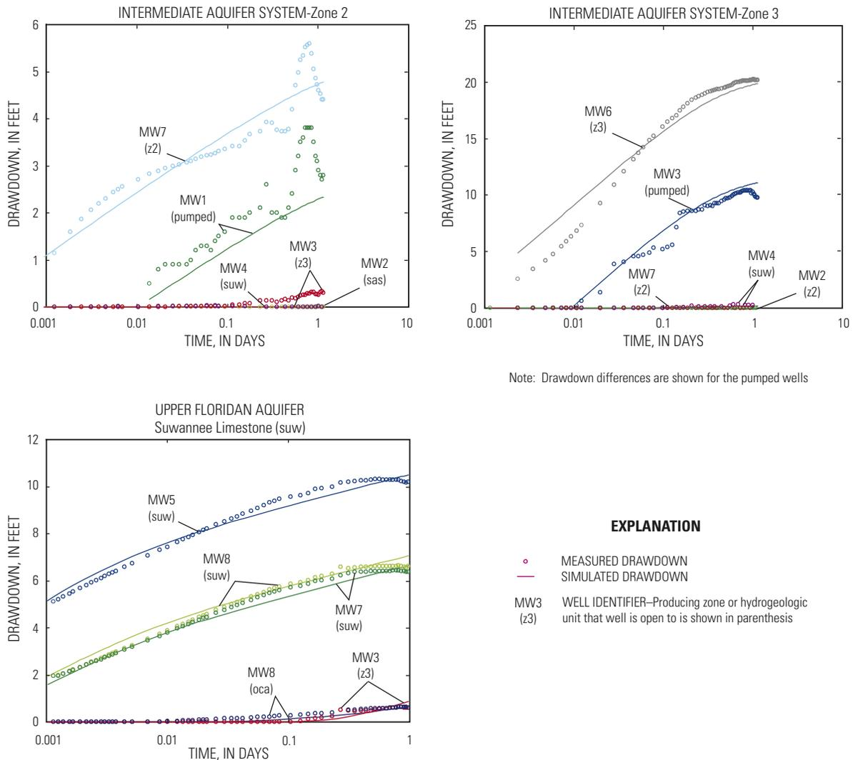
Figure 25. Simulated and measured drawdown for the three aquifer tests conducted at the ROMP 20 test site.
