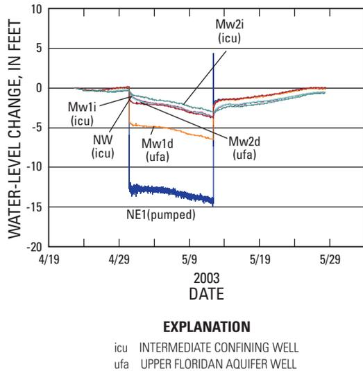
**Figure 46.** Water levels in selected wells during drawdown and recovery periods of the Upper Floridan aquifer test conducted at the Lakeland Northeast Well Field test site.
