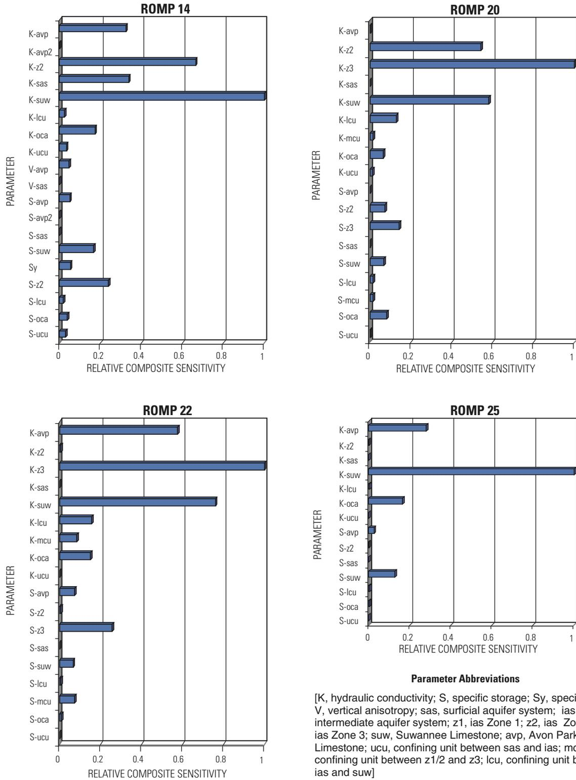
Figure 22. Relative composite sensitivity for final parameter values for ROMP 14, 20, 22, and 25.
