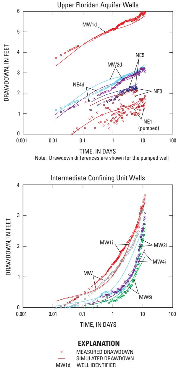
**Figure 47.** Simulated and measured drawdown for the Upper Floridan aquifer test conducted at the Lakeland Northeast Well Field test site.
